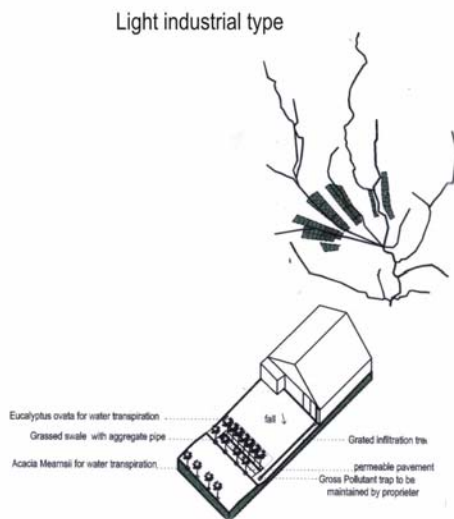
Figure 11 - Light industrial typology in Heath Gifford's Project for "the Floppy Studio" (Heath Gifford)
